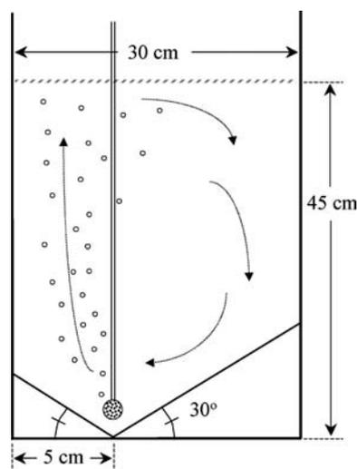
Figure 3. Schematic of the internal loop air-lift bioreactor used to study suspension and mixing intensity. The air-lift exterior is a glass tank with bottom baffling constructed of plexiglass (poly-methyl methacrylate) and sealed in place with silicone glue. Sparging was through two 0.2 μm HPLC mobile-phase spargers (Supelco, Bellefonte, PA). Off-center sparging and baffling geometry was based on previous studies to achieve high mixing with low gas flow rate.
