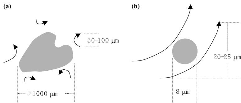
Figure 4. Schematic to depict the microscopic flow patterns calculated as the Kalmogorov eddy length (Equation (8)). For somatic embryos (a) the power level is based on minimum required for suspension of 3.2 mm polystyrene beads in air-lift and stirred tank vessels; for yeast (b) the power level is a typical high-intensity stirred tank fermentation.
