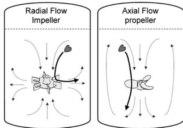
Figure 5. Implications of impeller flow patterns on 'inertial flow' and impeller impact on plant aggregates. Radial flow impellers draw flow inward from above and below with discharge towards the wall. Axial flow propellers push flow along the axis of the impeller shaft. Solid arrow represents typical embryo flow path through the impeller zone.
