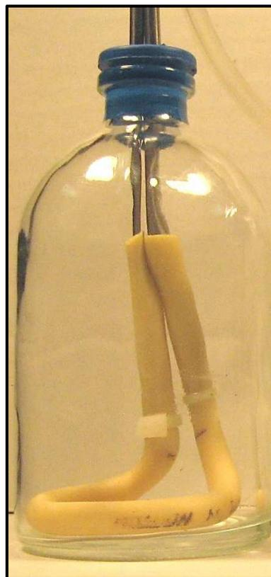
Figure 1. Anaerobic serum bottle fitted with 10 cm neoprene tubing for diffusive oxygen transfer. From [1].
