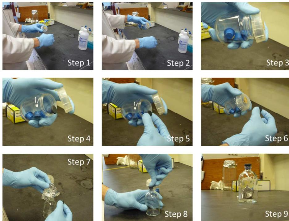
Figure 4. Procedure for placing stopper on anaerobic serum bottle.
