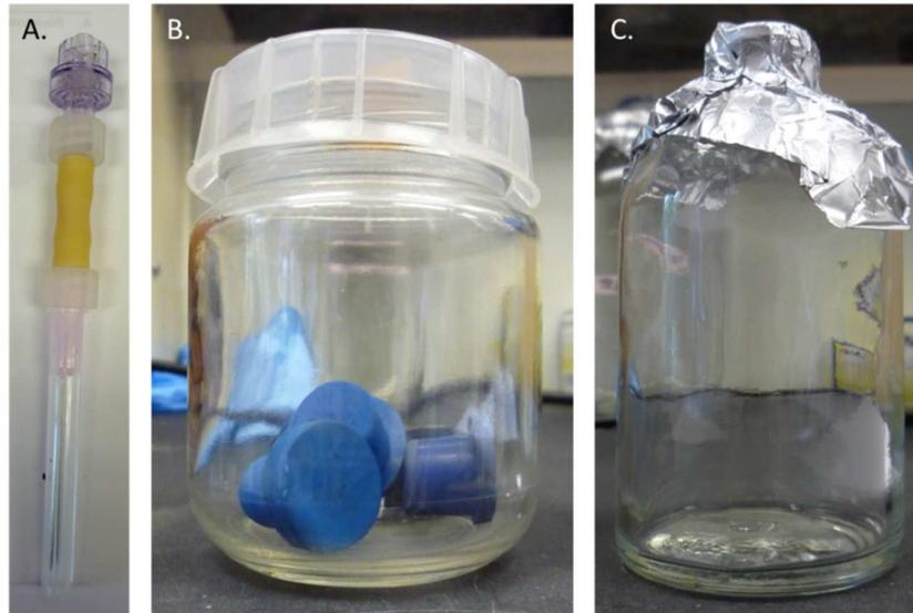
Figure 3. Supplies needed for inoculation. Gas release valves (A.), stoppers (B.) and serum bottles (C.).
